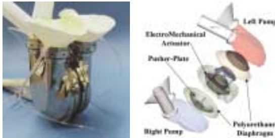
Fig. 11. Tokyo Medical and Dental University TAH (left) and its assembly diagram (right).
