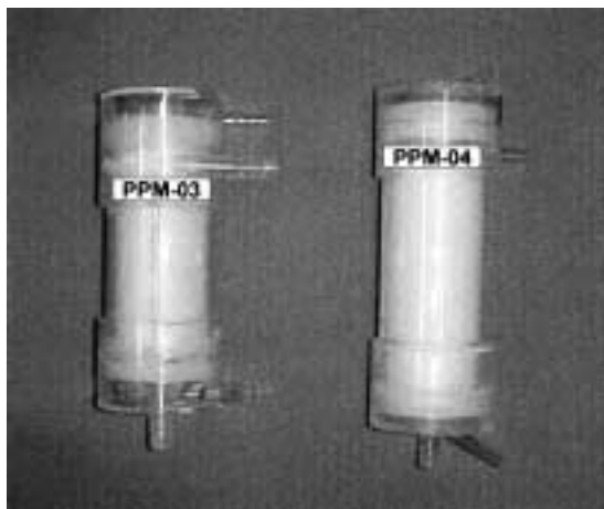
Fig. 2. The photograph shows the prototype silicone hollow fiber membrane oxygenators designed for ECMO (PPM-03 and PPM-04).
